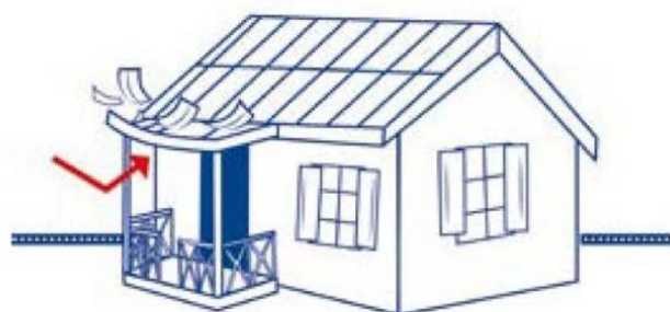
Smaller attached structures, such as verandahs and garages, can be easily damaged by high winds, as they may not be given the same level of attention during construction, and may not be properly secured
