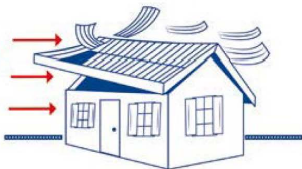
Cyclonic winds can also remove the roof framing and sheeting if not properly connected to the walls
